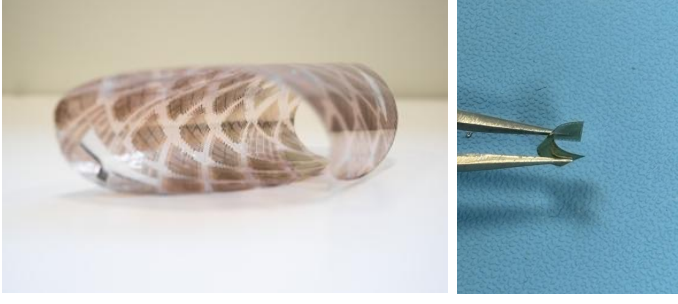
Fig. 1: A flexible wafer on a polyimide substrate, and a FlexIC held in a tweezer
